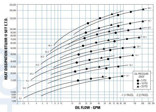
Performance Curves are based on 50 SSU oil entering the cooler  $50^{\circ}$ F higher than the ambient air temperature used for cooling. This is referred to as a  $50^{\circ}$ F E.T.D.
