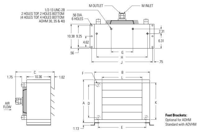
See dimensional chart for external NPT or optional internal SAE connection size.
